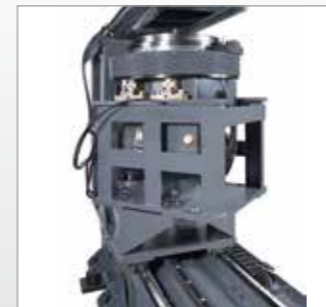
/ RACK & PINION STRUCTURE OF MILLING HEAD STORAGE
