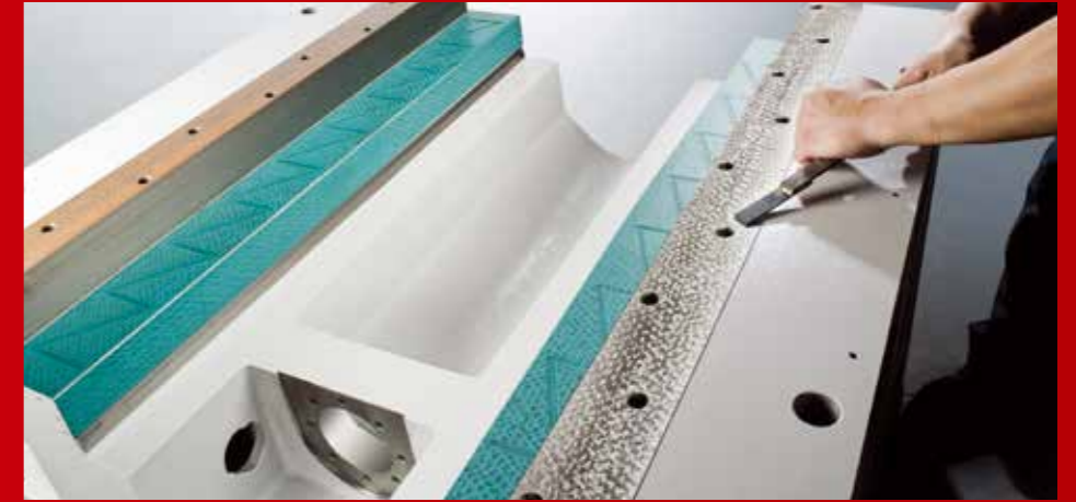
• Scrapping-The difference from other brand, with the KAFO line of Machining Centers, every component surface is finished by hand-scraping for a proper fit, ensuring that the machine itself is geometrically correct and long lasting. The hand-scraping process is labor intensive and must be performed by skilled craftsman who are trained in the technique. Machine components must be placed then removed up to 5 times to confirm that the machine base in both level and square.
