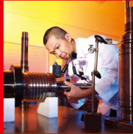
• Spindle assembly and adjustment in clean room with constant temperature and humidity.
