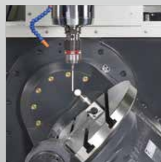
/ BLUM TC-50 infrared probe for automatic kinematic measurement and calibration of 5 axis positioning.
